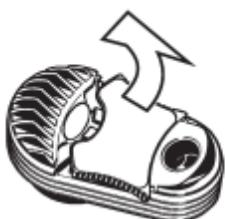
When cleaning the Cooling Unit Cap in isopropyl alcohol, remove the cap lock by pulling it up on one side.
