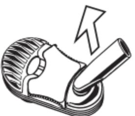
Pull the Mouthpiece out of the Cooling Unit Cap while slightly tilting it back and forth.
