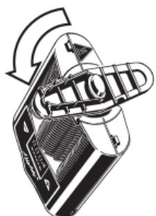
Unscrew the Cooling Unit base from the Vaporizer by turning it 90° counterclockwise.
