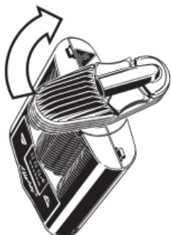
Screw the Cooling Unit onto the Vaporizer by turning 90° clockwise.
