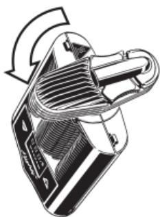
Unscrew the Cooling Unit from the Vaporizer by turning it 90° counterclockwise.
