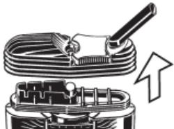
Pull the Cooling Unit Cap off the Vaporizer.
