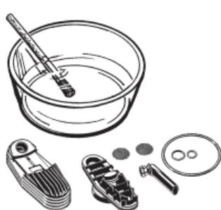
Place all parts of the Cooling Unit in warm rinsing water.
