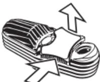
When cleaning the Cooling Unit Cap in isopropyl alcohol, remove the cap lock by pulling it up on one side. First press the cap lock on one side and pull it up on the opposite side.
