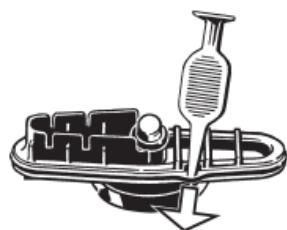
Lever out the large Base Seal Ring with Filling Chamber Tool at the recess in the groove.
