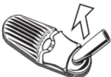
Pull the Mouthpiece out of the Cooling Unit Cap while slightly tilting it back and forth.
