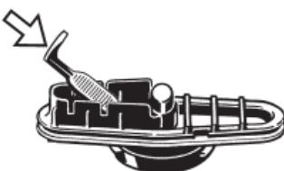
Press the Screen with the Filling Chamber Tool from the top to the bottom out of the Cooling Unit base.
